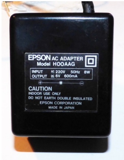
Figure 1: The original power supply unit says “6 V” on the label.
